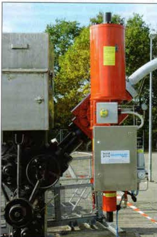
Fig. 3 Quick-closing safety valve installed at wellhead
