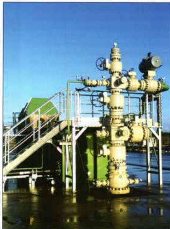
Fig. 1 Typical wellhead setup for a gas storage cavern
