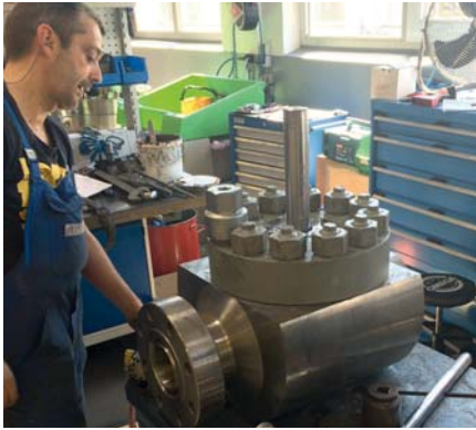
Overhauled ball valve (4 1/16" PN 520) during re-assembly at the Hartmann factory.
