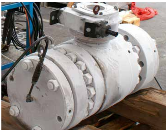
Hartmann's high-performance valves at cryogenic testing and fire safe.
