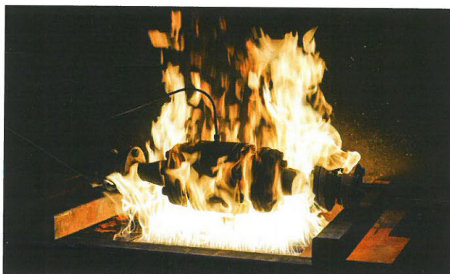
Fire-Safe testing is a standard for high performance valves.
