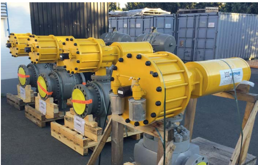
The refurbished safety ball valves are ready to be returned.
