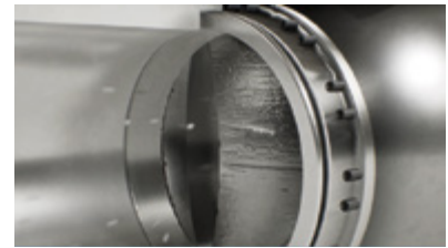
Embedded particles lead to scratches on the ball.
