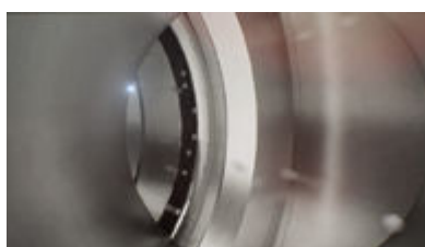
The soft seal is damaged on the downstream side.
